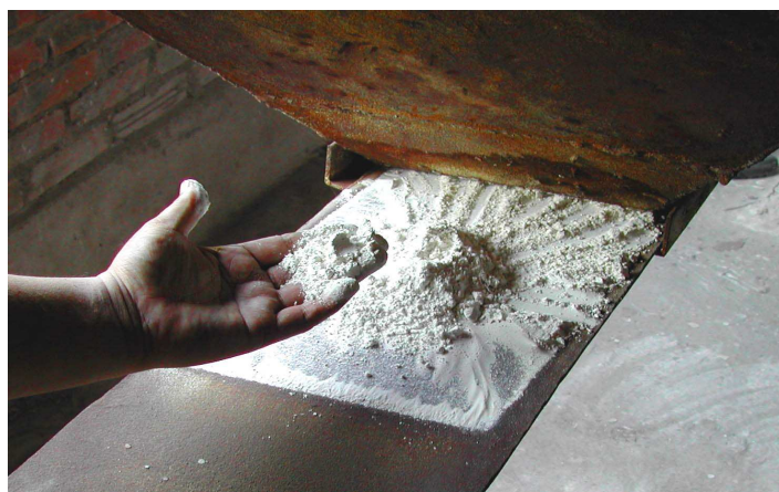
Figure 13a-c : Impressions from the central Cam Pha antimony central smelter with crude antimony trioxide end product
